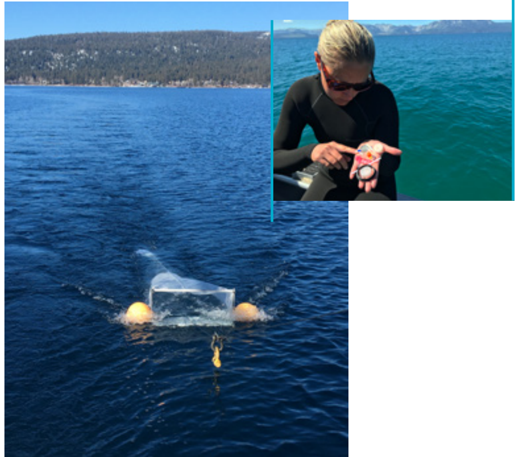
Manta net trawling for microplastics in 2020 while researcher Katie Senft reviews some of the macroplastics found in a trawl sample (inset).
